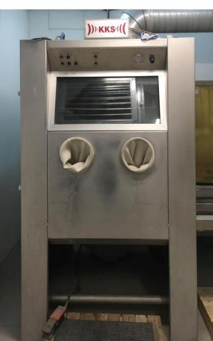
Our service department equipped with all necessary tools, lifting machines. Wet blasting machine and ultrasonic bath let us make careful cleaning of contaminated parts.
